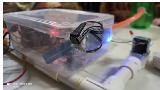
Fig 5a: shows the connection between the observatory kit and the DTMF module.
