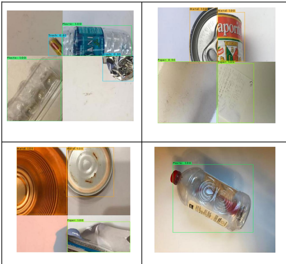
Fig.5. Example YOLO -v4-tiny predictions for TrashNet waste datasets
