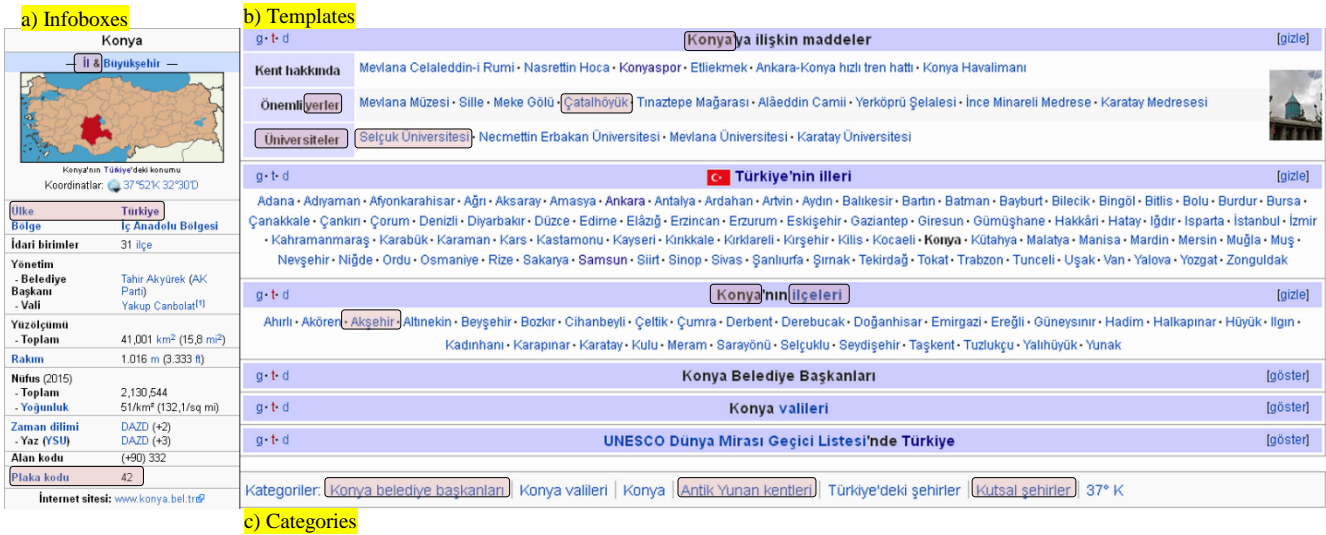
Figure 2. Components of Wikipedi Konya article: a) A city infobox b)Templates c)Categories. The parts marked show the places where ontological relations of Table 1 can be extracted from.
