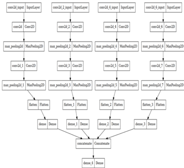
Fig. 14. CNN architecture for Three modalities in Late Fusion
