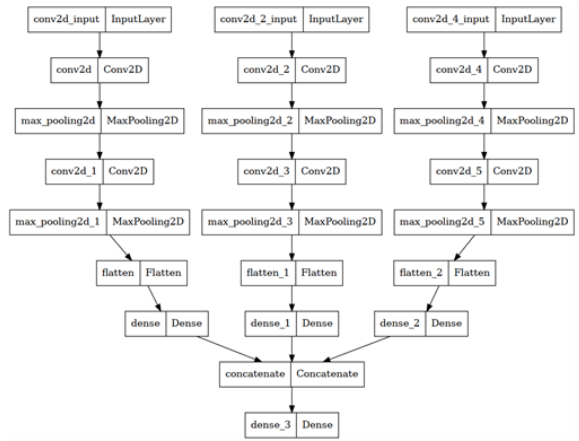
Fig. 15. CNN architecture for Four modalities in Late Fusion
