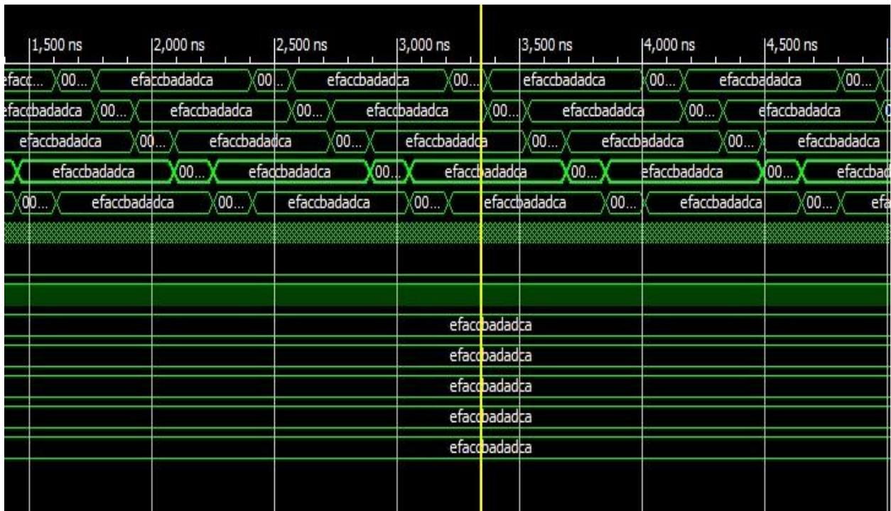
**Fig 4.** Simulated results of packet delivered at destination router
