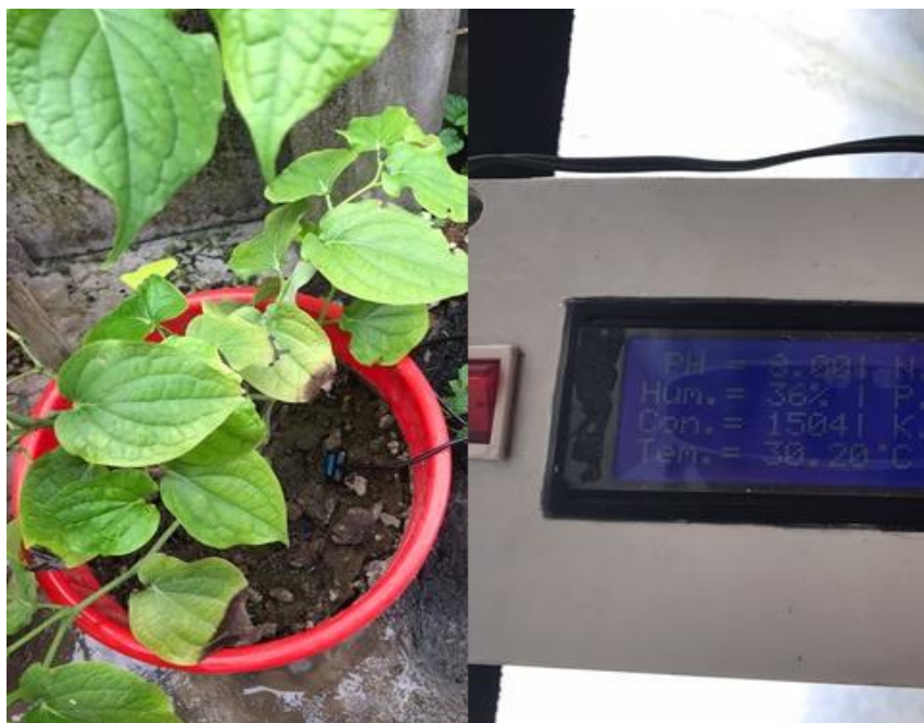
Fig 10: Showing results of Temperature and Moisture
