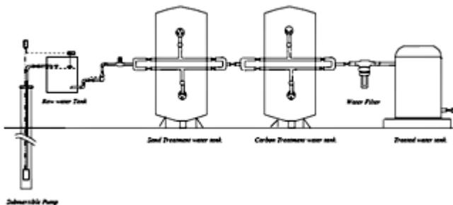
Fig 1.1. Flow sheet of a Simple water treatment plant.
