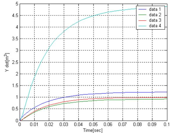
**Fig 1.4.** Effect of Restriction to flow on the Process, with  $R_1=0.5$
