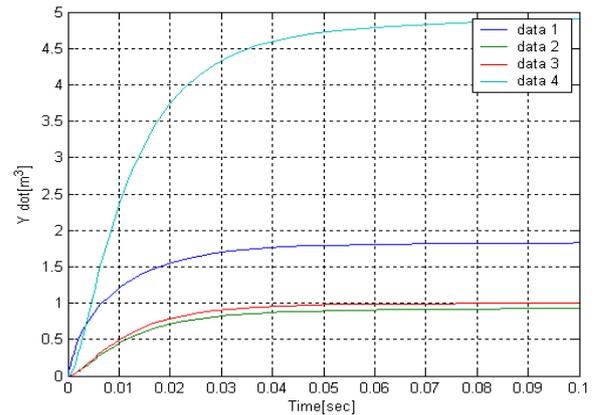
Fig 1.24: Effect of the Capacity of tank on the Process, with  $C_1=3e-03$
