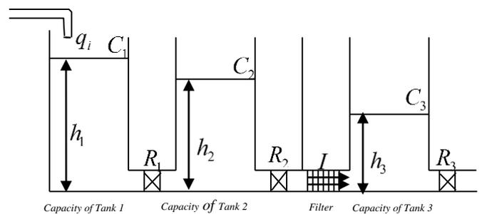
Figure 1.2. Coupled tank flow System.
