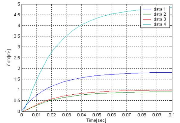
Fig 1.31. Effect of the Capacity of tank on the Process, with  $C_2 = 7e-03$
