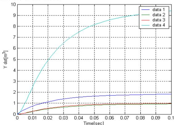
Fig 1.33. Effect of the Capacity of tank on the Process, with  $C_3 = 1000e-03$
