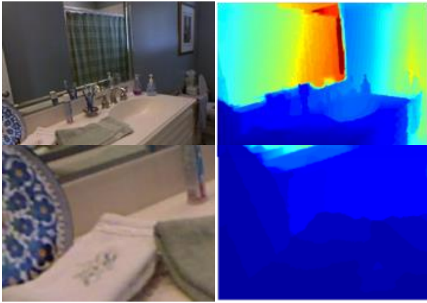
Figure 2. An example RGB and depth image pair from NYU-Depth v2 Dataset [24]. The boundary of the white towel on the bathroom sink is not visible in the RGB image, but is apparent in the depth map (Best viewed in color).
