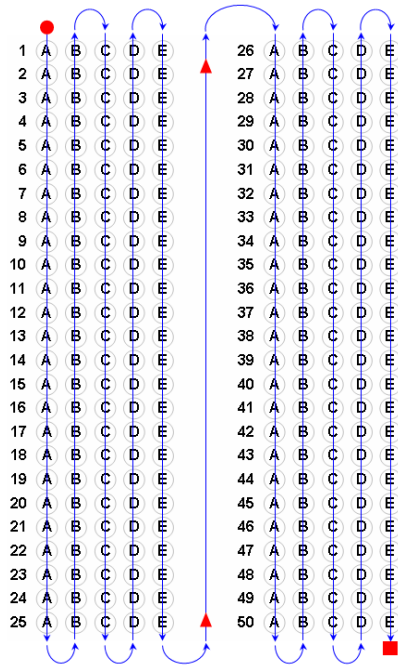
Figure 9. The illustration of the guidance system for the circle detection procedure in case the answer sheet has two columns and 2x25 questions. The starting and finishing points of the detection are indicated by red-filled dot and square, respectively. The crossing from one column to the next is shown by red-filled triangle
