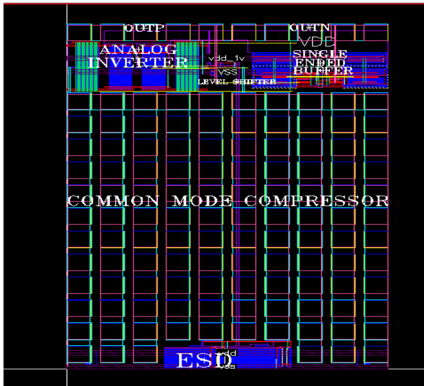
Fig 14: Layout Design of LVDS Receiver architecture
