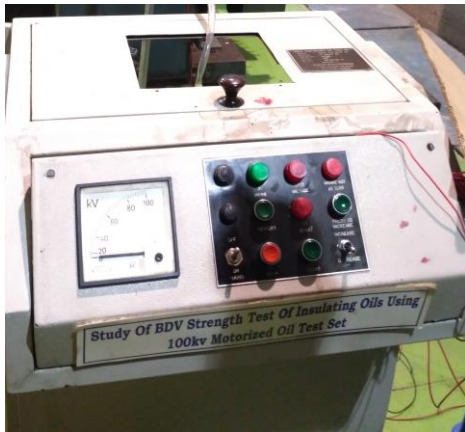
Fig. 1. Breakdown Voltage test kit.
