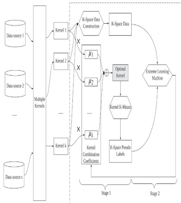
**Fig 3.** Design of TUMK-ELM for heterogeneous data processing [2]
