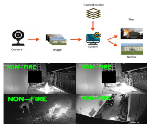
Fig 5. Fire detection system
