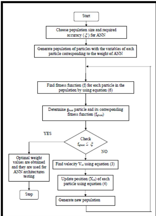
**Fig 1.9-** ANN training and testing flow chart using the PSO algorithm
