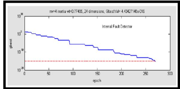
**Fig 1.15 .** The convergence curve for the WNN-scheme trained on PSO (IFD)
