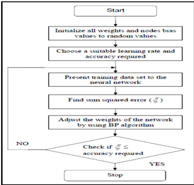
**Fig 1.8.** ANN Training and Testing Flow Chart using the BP Algorithm
