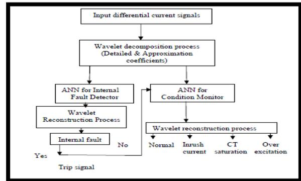
**Fig 1.12.** Diagram showing the planned WNN scheme's flow.
