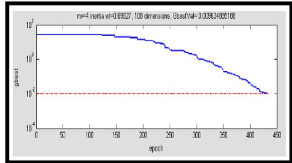
**Fig 1.16 .**Convergence curve for PSO trained WNN scheme (CM)
