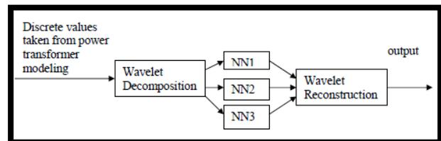
**Fig 1.13** Three stages of the proposed protection model (WNN)
