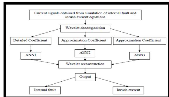
**Fig 1.3.** Flow diagram for the designed neural-network and wavelet-transform integrated power transformer protection scheme
