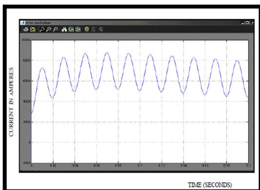
Fig 1.5 (c) Operating under Over-excitation condition
