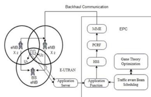
**Fig. 1.** LTE-A Architecture for 5G Communication
