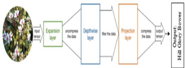
Fig 7. MobileNetV2 deep learning model architecture.
