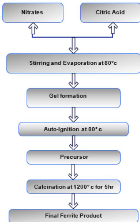
Fig.1 Flow Chart of Solution-Gel Auto Method
