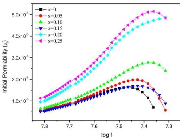
**Fig.8** Initial permeability with frequency for  $\text{Ni}_{0.7}\text{Mn}_{0.2}\text{Cu}_{0.1}\text{Fe}_{2-x}\text{Al}_x\text{O}_4$  The value x ranges from 0, 0.05, 0.1, 0.15, 0.2, and 0.25
