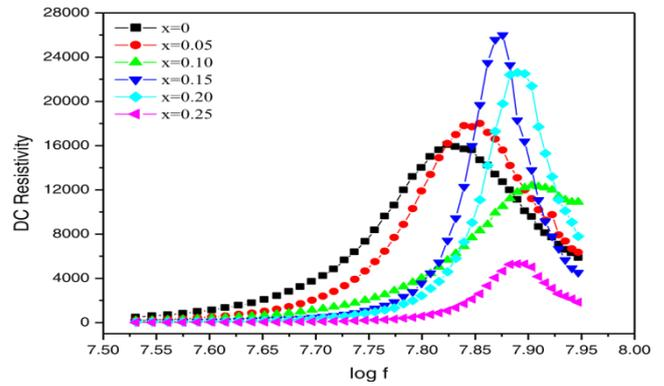
**Fig.6**  $Ni_{0.7}Mn_{0.2}Cu_{0.1}Fe_{2-x}Al_xO_4$  The value  $x$  ranges from 0, 0.05, 0.1, 0.15, 0.2, and 0.25 with respect to resistivity & frequency
