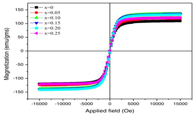
**Fig.7** M-H Loop for  $Ni_{0.7}Mn_{0.2}Cu_{0.1}Fe_{2-x}Al_xO_4$  The value  $x$  ranges from 0, 0.05, 0.1, 0.15, 0.2, and 0.25
