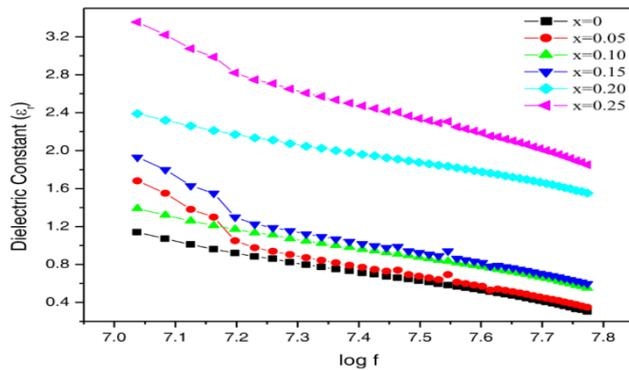
**Fig.4**  $Ni_{0.7}Mn_{0.2}Cu_{0.1}Fe_{2-x}Al_xO_4$  The value of  $x$  ranges from 0, 0.05, 0.1, 0.15, 0.2, and 0.25 with respect to  $\epsilon_r$  & frequency .
