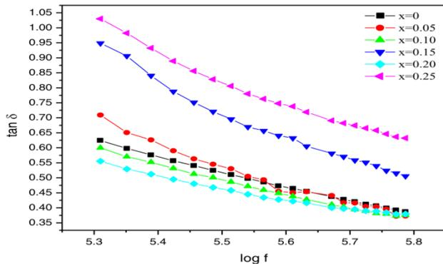
**Fig.5.**  $Ni_{0.7}Mn_{0.2}Cu_{0.1}Fe_{2-x}Al_xO_4$  the value  $x$  ranges from 0, 0.05, 0.1, 0.15, 0.2, and 0.25 with respect to  $\tan \delta$  & frequency.
