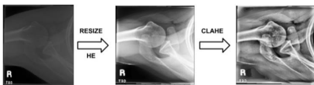
Fig. 2. Transformation of the image using HE and CLAHE
