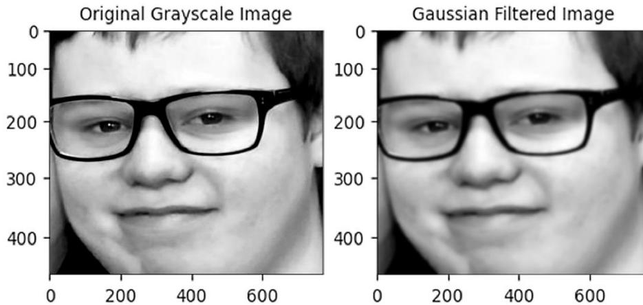
**Fig. 7.** Original Grayscale and Gaussian Filtered Image
