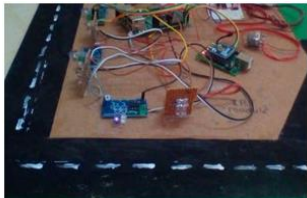
Fig. 10: Turn off the LED in the absence of a vehicle or object at low light intensity for node 2.
