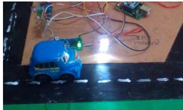
Fig. 9: Turn on the LED when a vehicle or object is detected at low light intensity for node 2.
