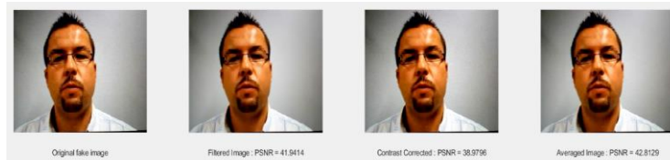
Fig. 5. The preprocessing stage. Original input image, Filtered image, Contrast corrected image, and the Averaged image. The PSNR values reflect pixel value changes in each stage.
