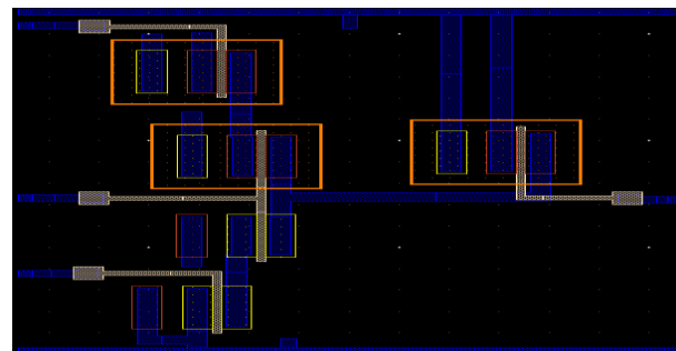
Fig.4.5 (b) Current starved based delay cell element layout.
