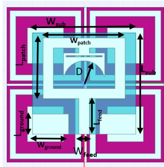
**Fig.1.** CPW-fed antenna design
