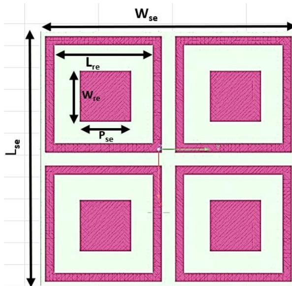
**Fig.2.** EBG Array Structure
