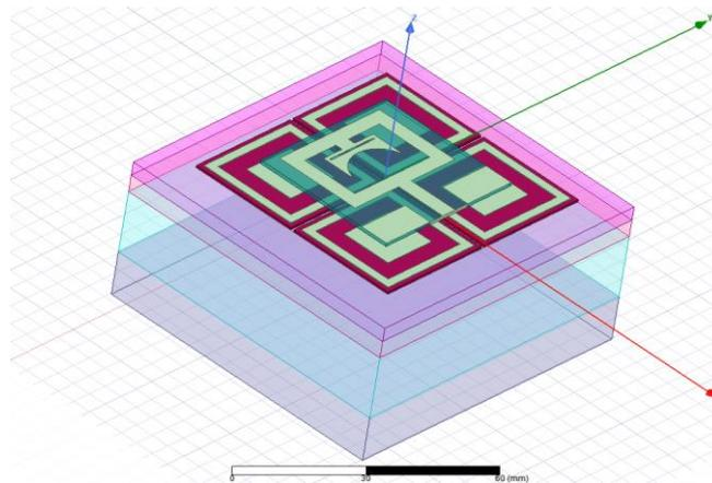
**Fig.5.** Electromagnetic Band Gap structure and a human body model.
