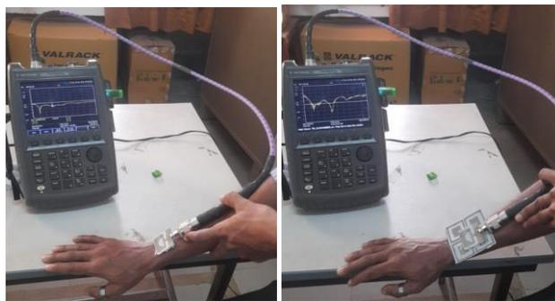
**Fig.7.** A fabricated integrated design positioned on the human arm.
