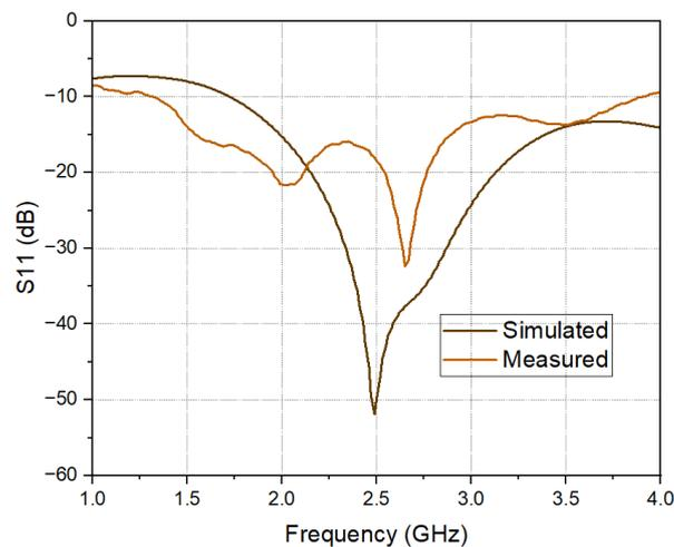
**Fig.8.** Simulated and measured reflection coefficient
