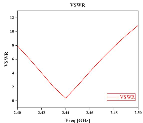
**Fig 4.** A measure of VSWR at 5mg concentration.
