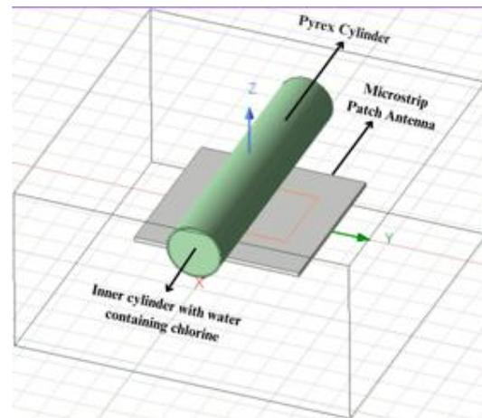
**Fig 2.** Representation of MPS with Tube.
