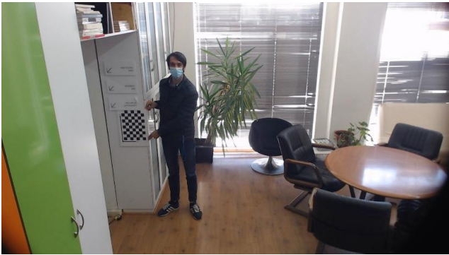
Fig. 13. Captured image for the calculation of the intrinsic parameters with the vanishing points in a controlled context.
