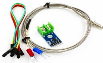
Fig. 2. Thermocouple K-Type and Module MAX6675
