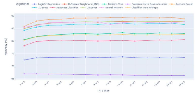
Fig. 6. Performance comparison of ML algorithms for respective Thepade SBTC Ary sizes for feature extraction of histopathology images in Cancer Detection
