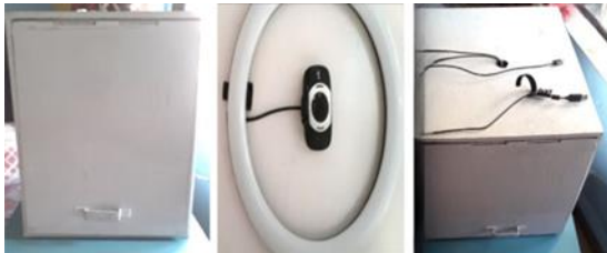
Fig. 5. Components of Multi-spectral Imaging Chamber (RGB LED Ring, USB Camera, Wooden Enclosure with Door).
