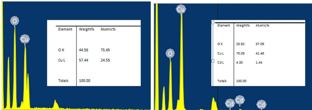
**Fig 3.** Chemical composition of CuO and CdO doped CuO nanostructure.
