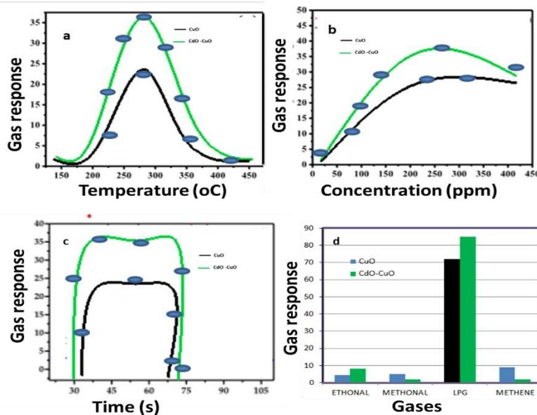
**Fig 4.** CuO and CdO doped CuO nanostructures gas sensing properties. a) operating temperature verses gas response, b)concentration verses gas response, c)response and recovery time verses gas response, d) gases verses gas response.
