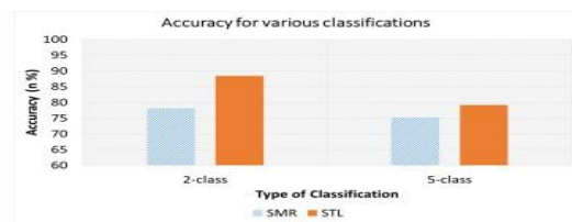
Figure 5: Classification accuracy using self-taught learning (STL) and soft-max regression (SMR) for 2-class and 5-class when applied to test data
