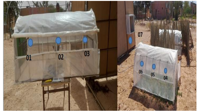
Fig. 7. Placement of Sensors in the two greenhouses
