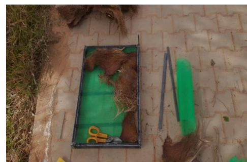
Fig. 4. Cooling system made of palm fiber
