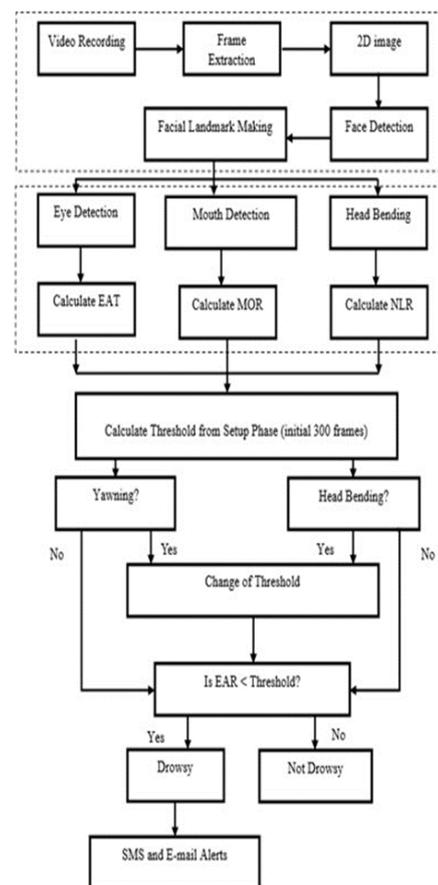
**Fig 8.** Proposed System Architecture of ASHS
