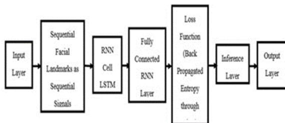
**Fig 6.** RNN Model architecture of ASH
