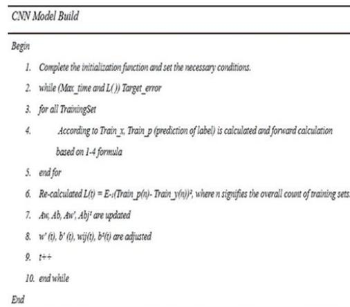
**Fig 3.** CNN Model Build Pseudocode
