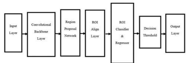
**Fig 4.** Faster Region-CNN Model architecture of ASHS
