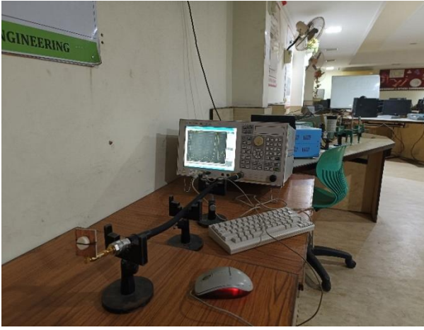
Fig. 18(b) shows the experimental set-up for measuring the parameters like resonant frequency, return loss and VSWR of the antennas
