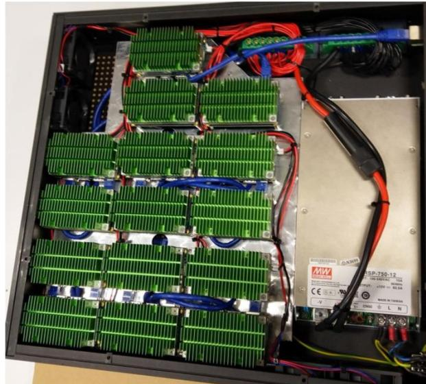
**Fig 5:** The 3U server vision sensor housing 15 NVIDIA Jetson TX2 modules, each which can handle one live video stream from security camera in real-time
