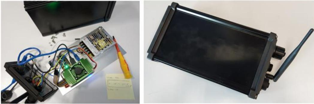
**Fig 2:** Inside and outside of smart visual sensor
