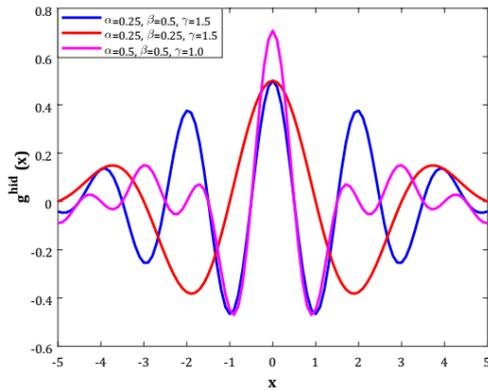
**Figure 2:** B-spline wavelet transfers functions with various values of  $\alpha$ ,  $\beta$ , and  $\gamma$
