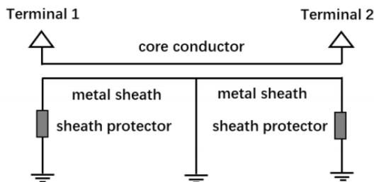
Fig. 6. Both-ends bonding method [34]
