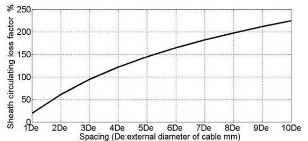
**Fig. 11.** Sheath circulating loss factor vs. conductor spacing (trefoil) [30]
