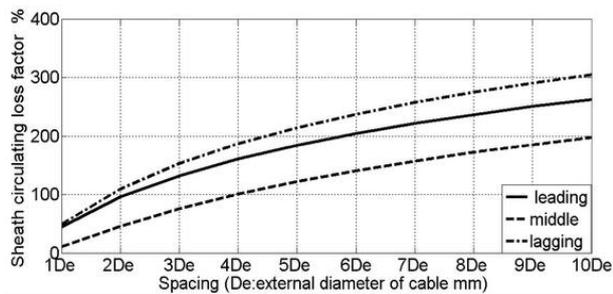
Fig. 12. Sheath circulating loss factor vs. conductor spacing (flat) [30]
