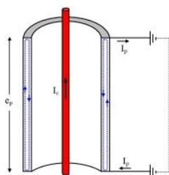
Fig. 2. Circulating currents in underground metallic sheath grounded at both ends [5]
