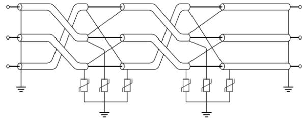
Fig. 8. Cross-bonding of cables with transposition [36]
