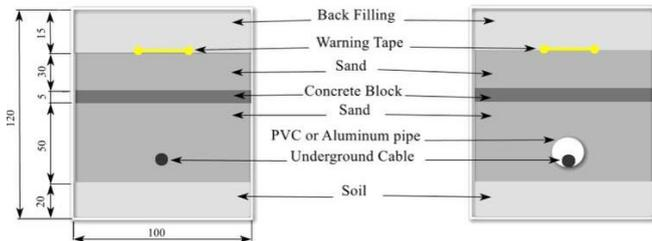
**Fig. 10.** MVUG cable laying conditions [10]
