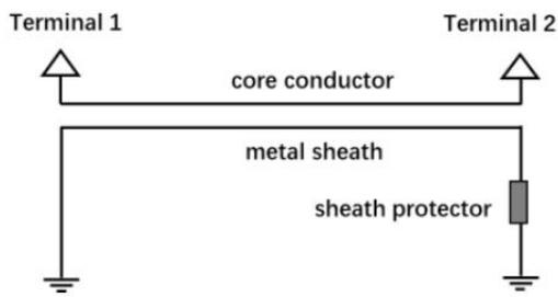
Fig. 5. Single-end bonding method [34]
