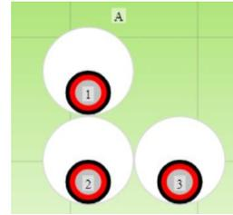
**Fig. 9.** Triangular formation of MVUG cables
