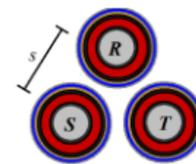
**Fig. 3.** 3-Core cables in trefoil formation [1]
