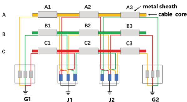
Fig. 7. Cross-bonding method [28]
