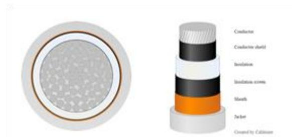
**Fig. 13.** Cross section of an 11kV MVUG cable conductor
