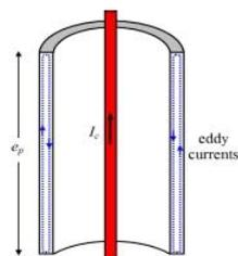
Fig. 1. Eddy currents in underground metallic sheath [5]
