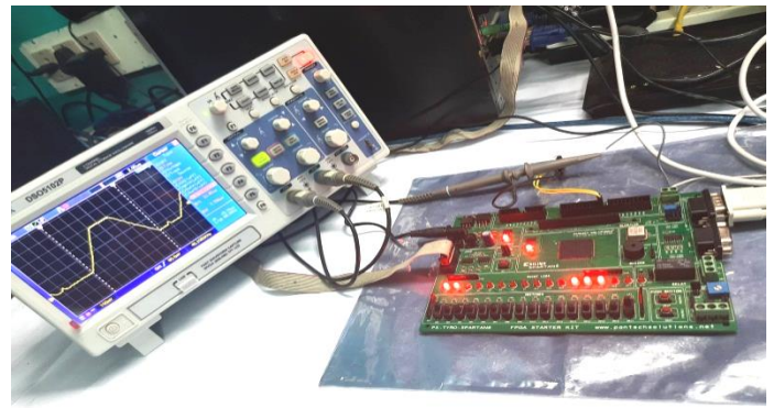
Fig 14 : Hardware Implementation setup and tested Noise Shaping ANS DAC Output in Oscilloscope
