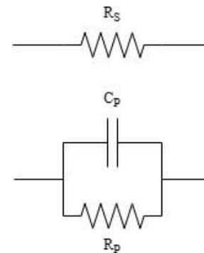
**Figure 2.** Equivalent circuit for PIN diode
