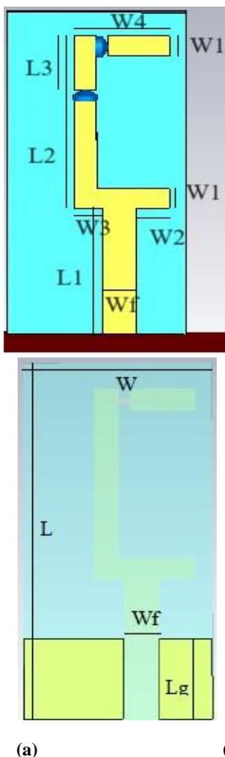
**Figure 1:** Geometry of antenna (a) top side (b) back side
