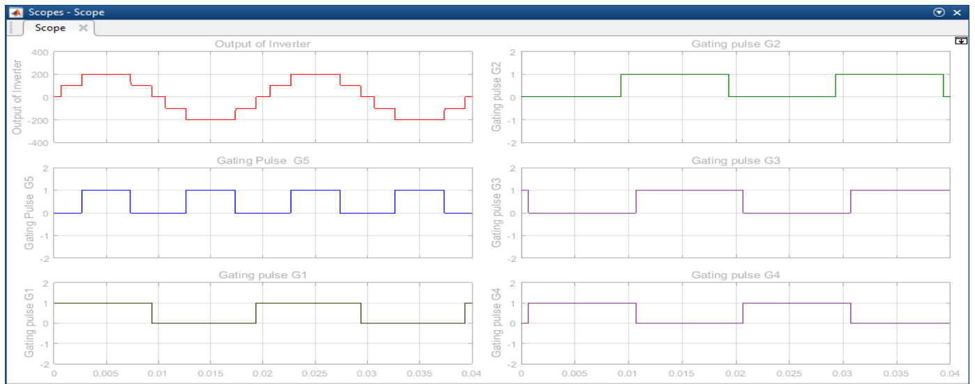
Fig.6 Simulink results of power circuit of single phase H5 topology and gating pulse generation
