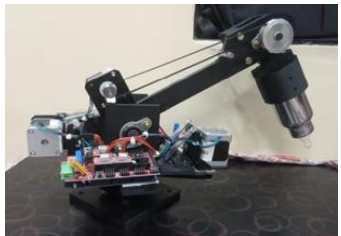
Fig.3. 3-Axis robotic arm to feeding the baby
