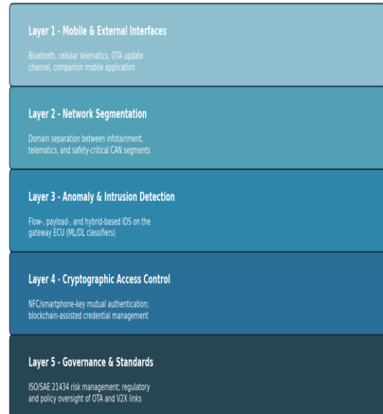
Fig. 4. Proposed five-layer reference architecture for secure mobile connected-vehicle platforms, synthesising mechanisms from Sections II through V.
