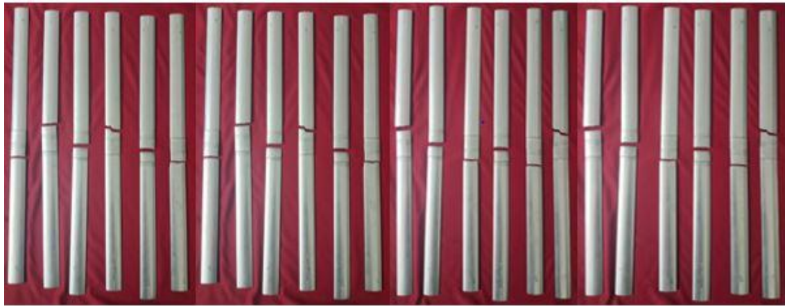
Fig. 22. Specimen after Tensile Fracture
