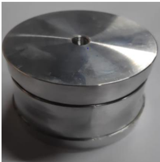
Fig. 10. Flyer-Target After Weld
