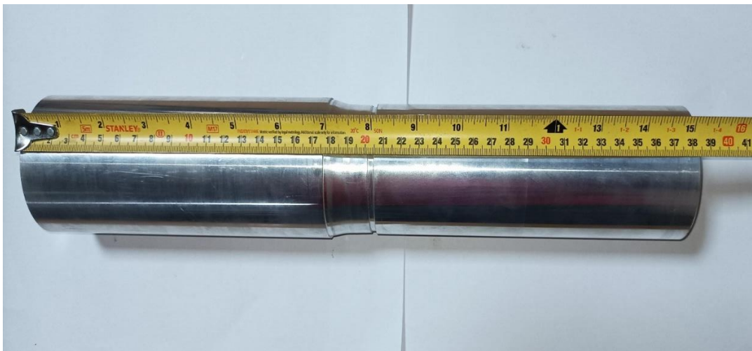
Fig. 15. Specimen after weld
