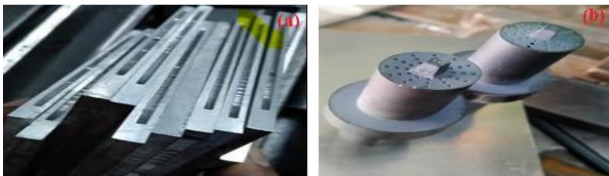
Fig 2. Processed materials across (a) Grooves prepared at joint interface for reinforcement materials (b) Square tapered tool used.
