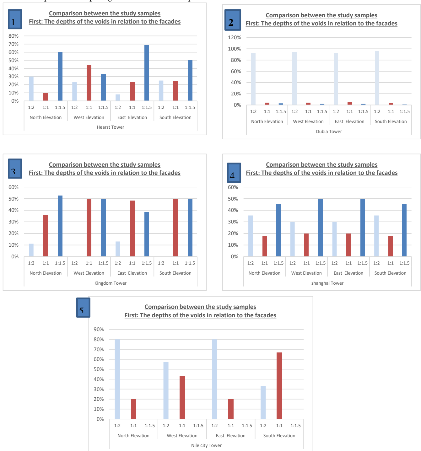
Fig 32. shows the depths of the voids in relation to the facades of the towers under study.
