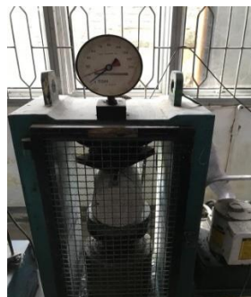
Fig 6. Split Tensile Strength Test Compressive
