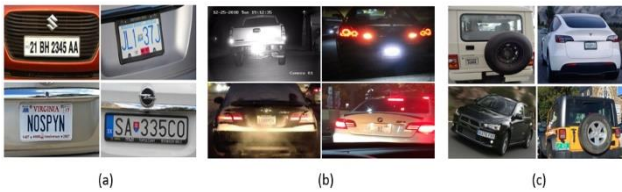
Fig.2 Some challenges in the LPR task. (a) License plates with different sizes, (b) The phenomenon of illumination and the subsequent reflection of headlights on license plates, (c) Different plate positions.
