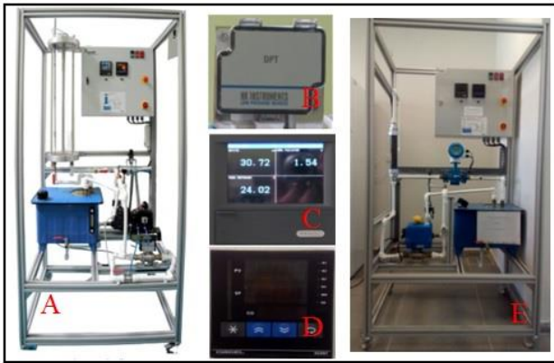
Fig. 1. a) LLCS, b) differential pressure sensor, c) recorder, d) process controller and e) FRCS
