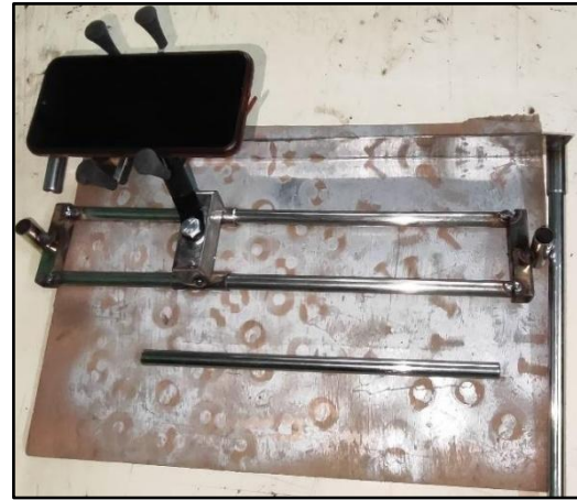
Figure 4 : Adjustable height and position for Camera Position in Upward –Downward direction and left right Direction
