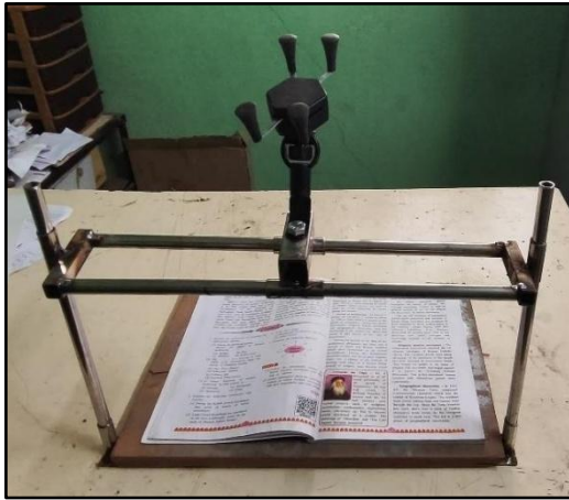
Figure 4 : Adjustable height and position for Camera Position in Upward –Downward direction and left right Direction
