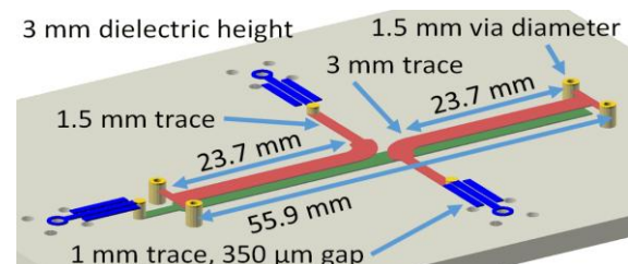
Figure 2: CAD view of a stripline Marchand balun with two stripline inner layers (green and red) and a top layer coplanar waveguide section (blue).
