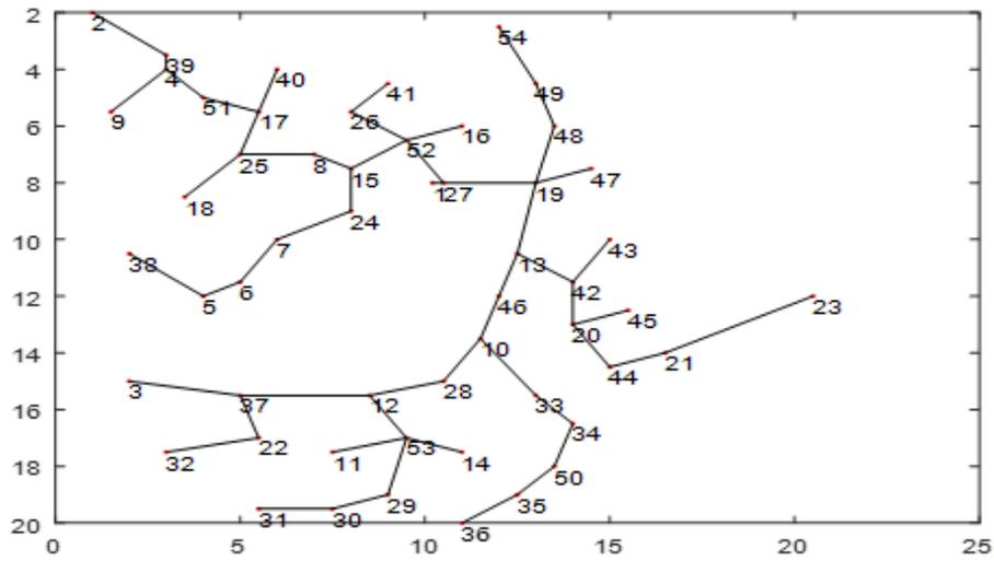
Figure 7. Optimal feeder configuration for single feeder
