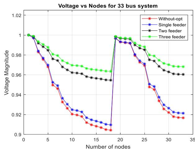
Figure 4. Voltage profile of 33 node radial distribution system
