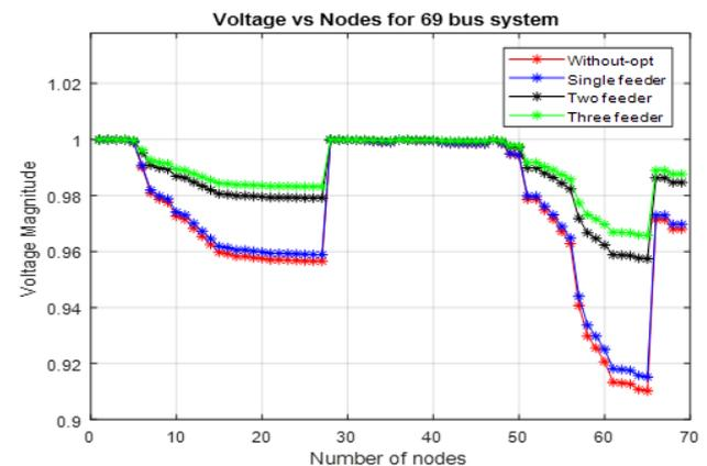
Figure 6. Voltage profile of 69 node radial distribution system
