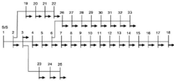
Figure 3. 33 node radial distribution network
