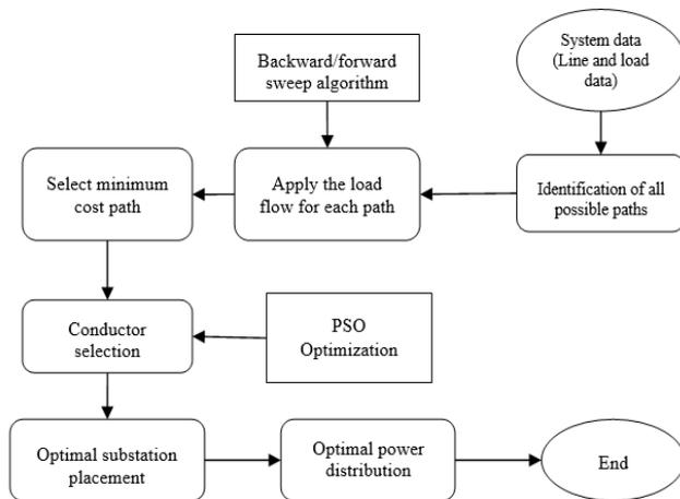
Figure 1. Block diagram of proposed optimal power distribution
