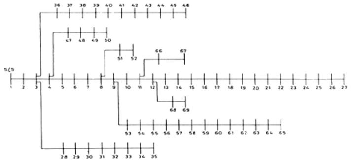
Figure 5. 69-node radial distribution network
